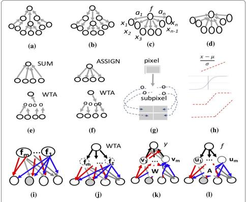
**Fig. 6** Basic mechanisms: PRODUCT, FAN-in/FAN-out, HIERARCHY, BOUND. **a** Converging causal tree. **b** Diverging causal tree. **c** Star topology collapsed from **b**. **d** Star topology collapsed from **a**. **e** FAN-in mechanisms. **f** FAN-out mechanisms. **g** Subpixel interpolation or mixture subpixel interpolation.**h** BOUND mechanisms. **i** Classical factor analysis (FA). **j** FA mix-star extension. **k** Forward neural networks. **l** backward neural networks
